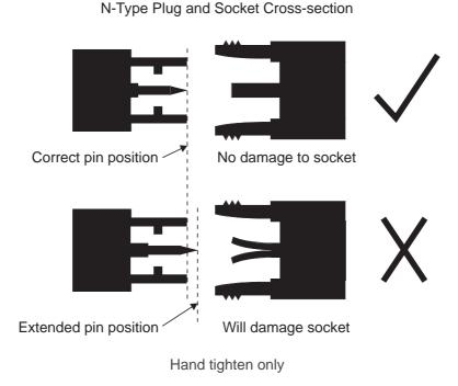
Figure 3.1 N-Type Plug Assembly Details
